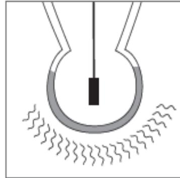
A proper cleaning and fresh solution ensures the whole surface of the sensor tip is reading correctly, ensuring an accurate calibration.
