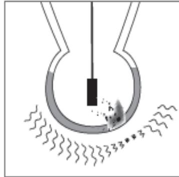
Your meter can still be calibrated even if the electrode sensor tip is not properly cleaned before calibration. If the contamination dissapates, the calibration is no longer valid and the readings are inaccurate.
