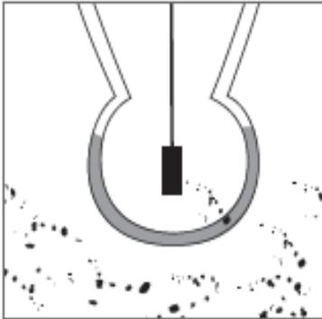
In time, particles during routine measurement can contaminate the sensor tip. Mishandled and aged solutions can also be affected.
